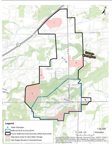
As part of the Water Storage Class Environmental Assessment, seven potential locations were identified within the Millbrook Settlement Area based on elevation, proximity to existing infrastructure and alignment with future development areas.
